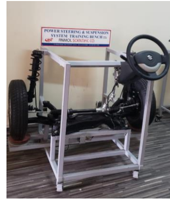
power steering & suspension system training bench
