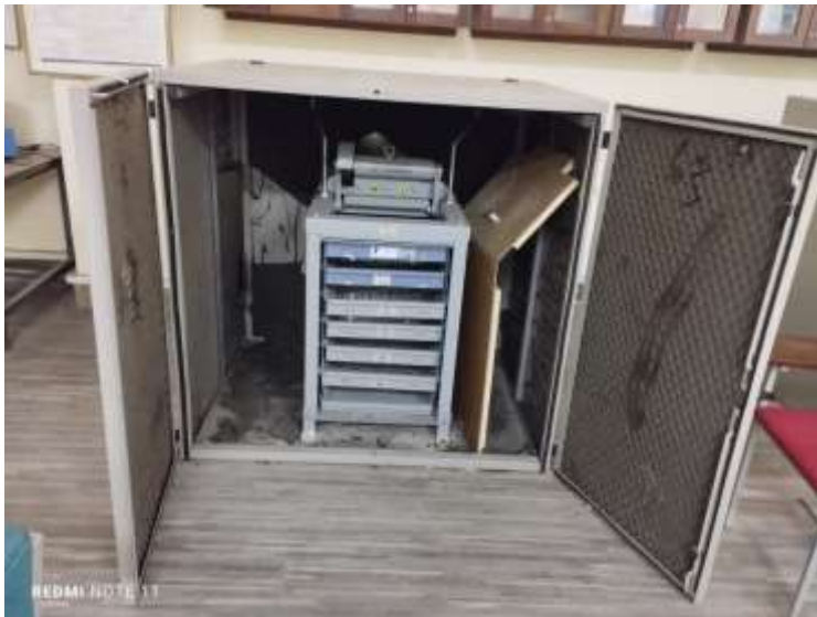
Aggregate Screen Shaker
