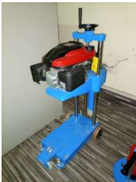
Pavement Core Drilling Machine
