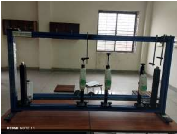
Deflection of Beams
