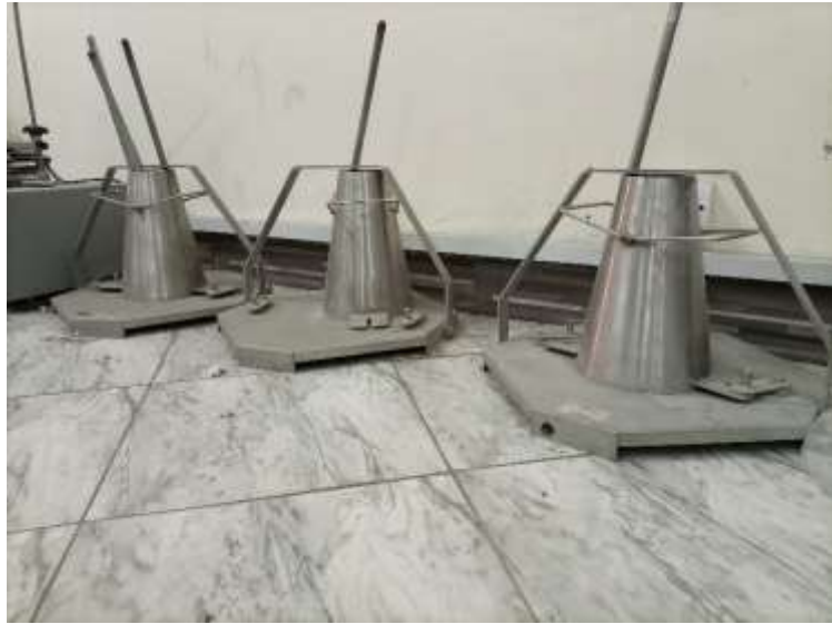
Concrete Slump Test
